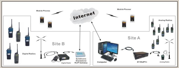
The Solidtronic ST-RoIP1+ RoIP PC-Radio Interface works with a PC to setup a RoIP gateway. It is developed to give the old PC a 2nd life to setup a RoIP gateway system for the interoperability between 2-way radio channel and Zello channel. Extends the 2-way radio communication everywhere.
